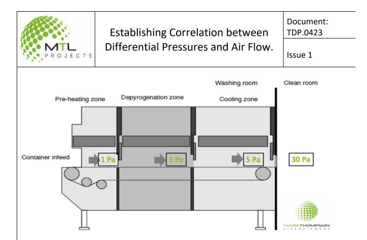
NOTE; Some Tunnels, particularly feeding isolators at higher pressure will have a sink pressure stage in cooling, possible 2 stage air lock.
